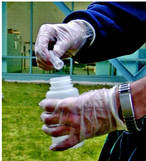
Photo 4. Handling and preserving of samples using safety gloves (Source: Environment Canada and B.C. WLAP (2005))
